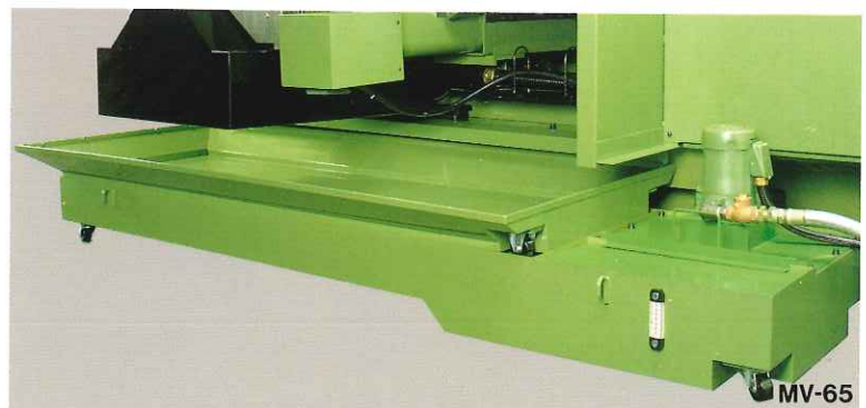
Large chip buckets on both sides of the machine. Optional chip conveyor improves chip disposal.
