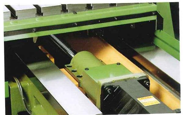
Special narrow guideways maintain linear precision.
