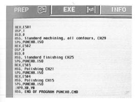
CT-Expert then selects the most appropriate wire (type and diameter) and the sequence of generator settings from roughing to finishing, and calculates the different offsets. And to recap things, the expert system generates the complete operational chain in the form of a command file.
